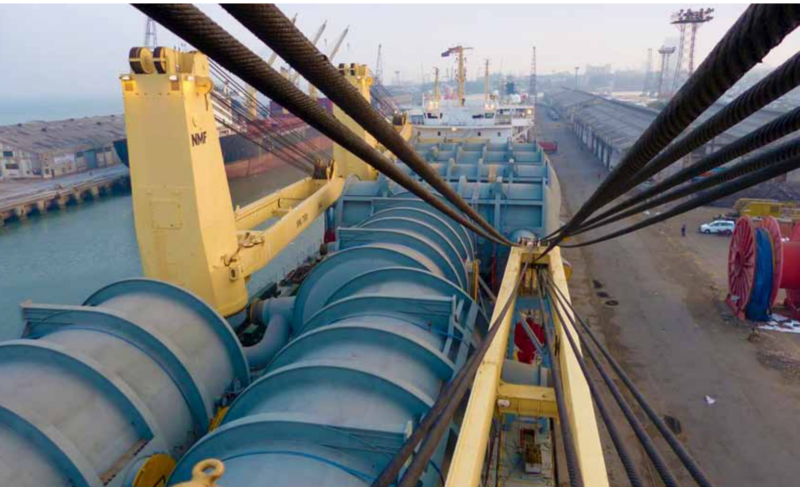
MV Anne-Sofie, deck fully loaded with Catofin Reactors (seen from crane 3)
