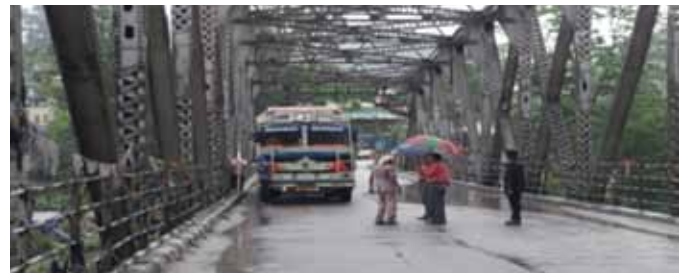
Fig 8: Stage-I Loading of Load Test on Rangpu Bridge (Taken From Sevoke, West Bengal side)
