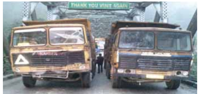
Fig 13: Stage-II Loading of Load Test on Rehabilitated Rangpu Bridge (Taken From Rangpo, Sikkim side)
