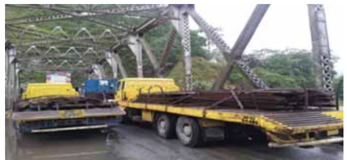
Fig 10: Stage-III Loading of Load Test on Rangpu Bridge (Taken From Rangpo, Sikkim side)
