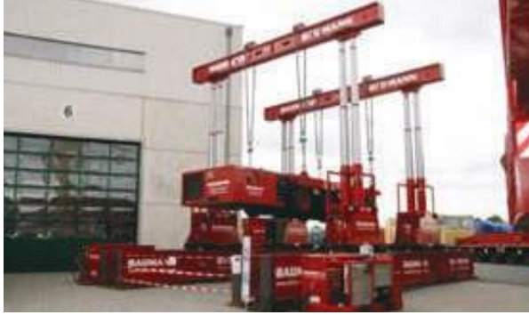
Figure 31. Telescopic bare lift cylinder.
