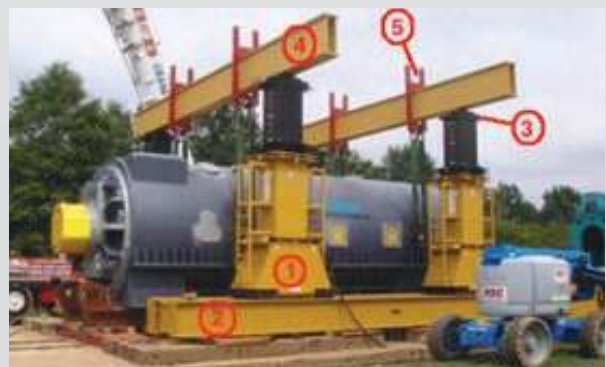
Figure 30. Telescopic gantry boom.
